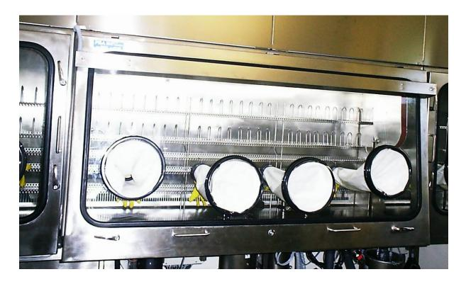
Production Isolator Connected to a Mixing Pressure Vessel
